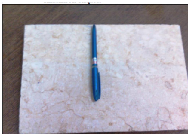
Fig. (2). One of the hand specimen of Shiekh Fadl hardened limestone.
